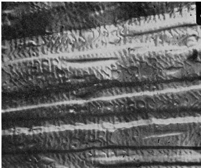
Fig. 7. Enlargement of fracture surface in Figure 6. The vertical striations represent crack hesitation points (27 \times ).
