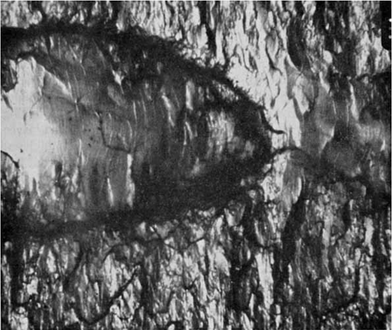
Fig. 9. Enlargement of fracture surface in Figure 8. The foot-shaped step is raised above the surface ( 27\times ).
